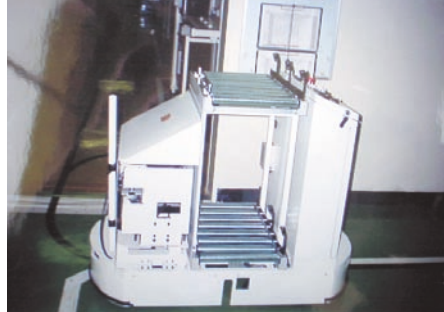
Powered roller material delivery and container return
