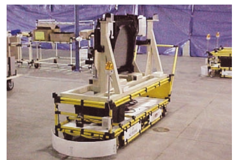
Mobile assembly line with part orientation fixture
