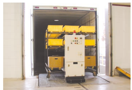
Custom designed AGC for automatic loading and unloading of trailers or trucks
